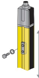
The **SLX-MO-CLIP** is used for fixed mounting of series SLC/SLD in device columns SLX-COL.
