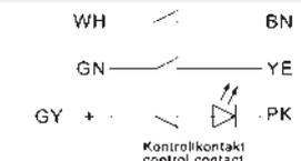
Contacts are shown in non-operated state (magnet is out of actuating distance Sar)
