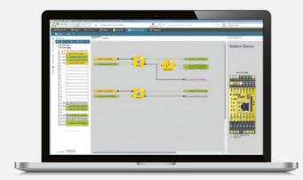
samos® PLAN 6 assists designers and machine builders with the programming, diagnosis, and documentation of all safety functions on a machine.
