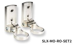
The swivel mount set **SLX-MO-RO-SET1** (**SLX-MO-RO-SET1S** with shock absorber) is used for wall mounting of Transmitter, Receiver and Transceiver from series SLD (240° horizontal adjustment possible).
