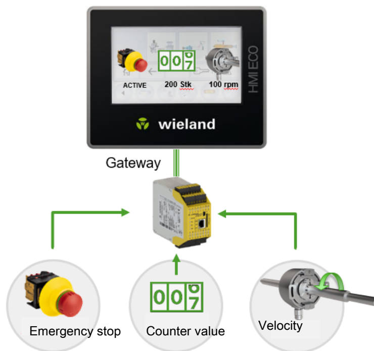
Fig. 8: Values via gateways to the HMI, PLC or the IIoT world
