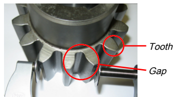
Fig. 207: An example of the toothed disc with tooth:gap ratio = 3:2.
