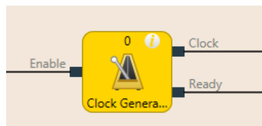
Fig. 67: Logical connections for the cycle generator function block
