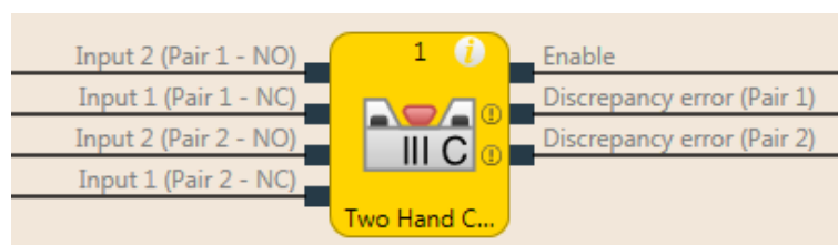
Fig. 125: Function block diagram for two-hand type IIIC function block
