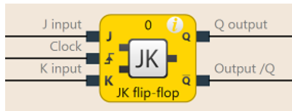
Fig. 66: Logical connections for the JK flip-flop function block
